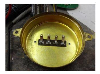
• Flip the tach sender over as we need to prepare and label the terminal strip. This step is very important. The tach will not work if the sender is wired up incorrectly. There is one modification required to the tach can. Note how the ground strap has been removed (you can leave it there not touching anything or you can pull it off and discard as we need to use this terminal ungrounded. In the new setup the tach can will be the ground so the ground terminal isn't needed
