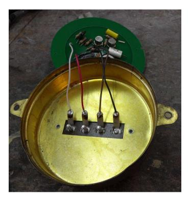
• Test fit the board into the sender can. Don't forget to line up the can and board via the notch and matching bump in the can. Mark the position alignment of the shiny solder pads on tach sender can.
