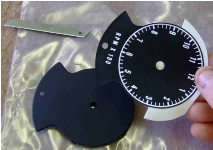
Figure 3. Applying a clock Decal (note how decal is held and all cutouts removed)
