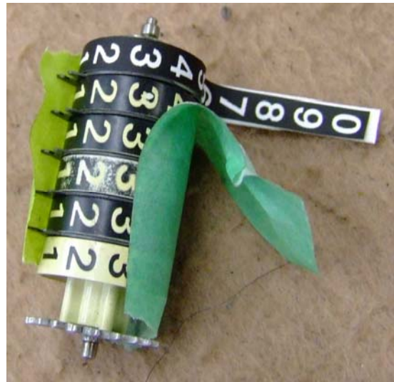
Figure 11. Using tape on 2 sides During Relabeling
