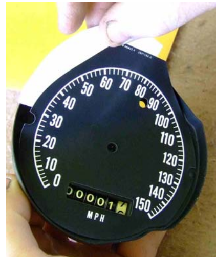
Figure 4. Applying a Speedo Decal (note how decal backing is used as a "handle" )
