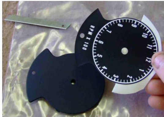
FIGURE 3 – Typical Installation technique using decal backing as a “handle” (B body tic toc clock shown)
