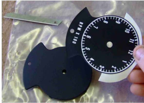
FIGURE 2 – Typical Installation technique using decal backing as a “handle” (B body tic toc clock shown)
